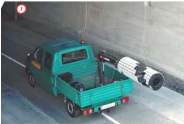
Figure 1 – Highspeed 3D system mounted on a crane
