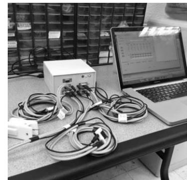
system used to obtain DVOS measurements.
