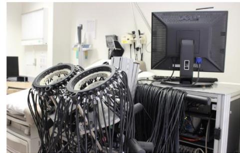
Figure 10 – Photograph of the custom-built diffuse optical tomographic breast imaging system (DOTBIS).
