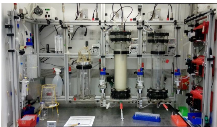
Figure 9: Experimental setup with stirred tank reactor and two 2 liter bubble column reactors for fermentative butane oxidation
