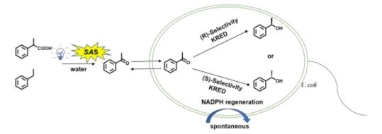
Figure 23 – Photochemo-enzymatic one-pot cascade in the whole-cell reaction system.
