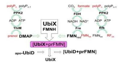
Figure 9 – Schematic diagram showing the in vitro cascade system for prFMN biosynthesis and UbiD decarboxylase. The system includes cyclic and linear (re)generation reactions for ATP, NADH, DMAP and FMN, as well as for enzymatic oxygen removal (FDH).
