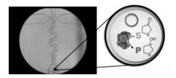
Directed evolution & semi-rational design of an ADH using ultra high-throughput droplet-based microfluidic screening of single cells.
