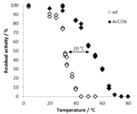
Figure 1. Improved thermostability of choline oxidase six-point variant compared to the wildtype.
