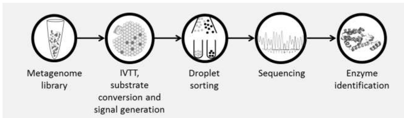
*Figure 1 Workflow of the all-in-one metagenome screening platform. DNA fragments of metagenome library are emulsified in micro droplets. Inside the droplet the *in vitro* transcription and translation (IVTT) takes place. Upon substrate conversion specific enzymes will generate a signal. Following droplet sorting the DNA sequence of active enzymes can be determined.*
