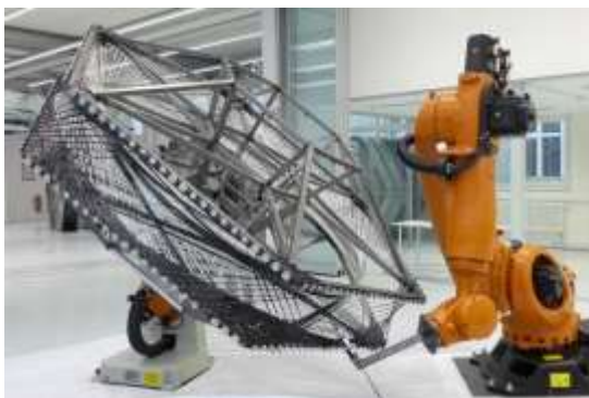
Figure 1 – Robotic filament winding of large-scale building elements
