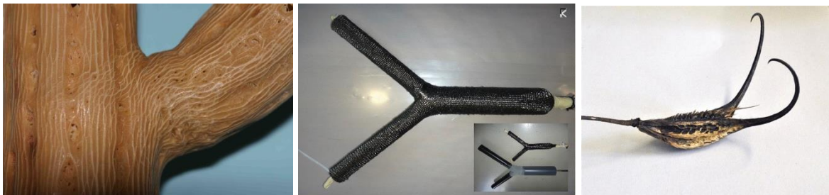
Fig. 1: the stem branch junction of columnar Cactaceae (left) served as model for a novel carbon fibre reinforced component in light weight construction (center). The fruits of Proboscidea (right) consist of sclerenchymatous fibres only, but exhibit superior mechanical properties und different load conditions.
