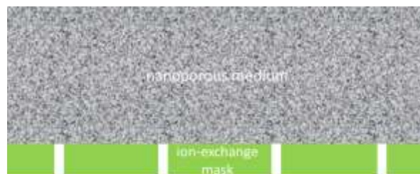
Figure 2 – Schematics of sandwiched nanoporous and micro-perforated ion-exchange layers
