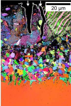
Figure 2 – Structure of a (Pt,Ni)Al coating after SPLCF cycling. Cracks are outlined in white.
